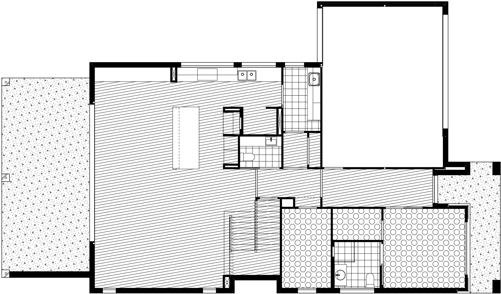
FLOOR COVERINGS (GROUND FLOOR) SCALE: 1:100
